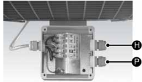
Fig. 13 - External junction box opened.
